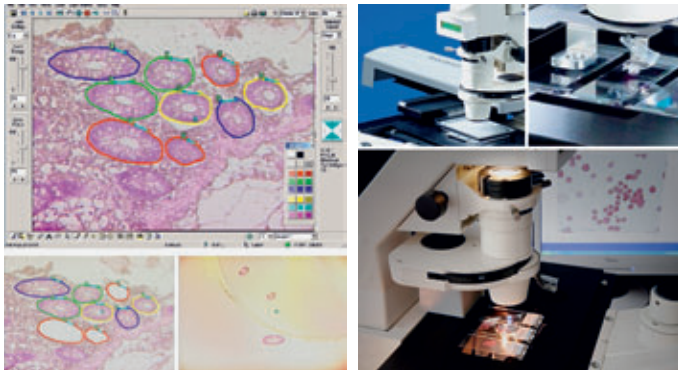
Figure 10: Colour-coded areas are catapulted accordingly; Robo-Mover and RoboStage enable improved sample capture with enhanced throughput (image lower right courtesy of Berthold Leibinger Foundation)
