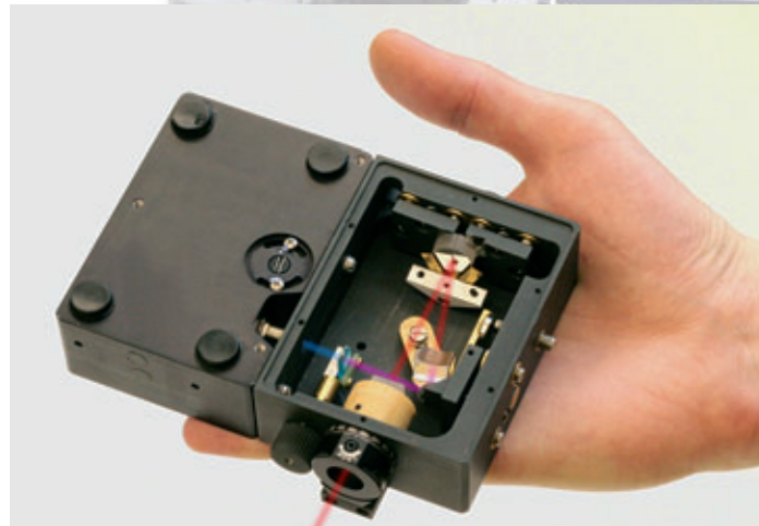
Figure 1: The latest generation of ultra-compact pulse characterisation devices can come in handy. A micro-SPIDER for measuring the 30 fs pulses from a standard Ti:Sapphire laser system is shown
